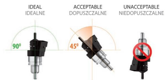
The way of reaming the injector nozzles
